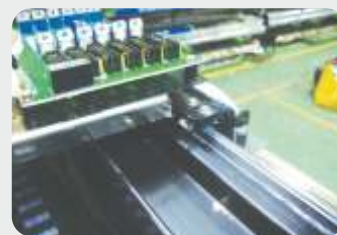
New Dust Proof Sealed Linear Bearings for High Speed Carriage Motion
